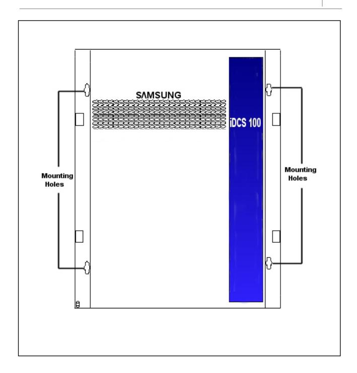
Figure 1–1 *i*DCS100 Basic Key Service Unit
